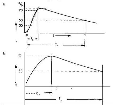
Fig. 4 Standardized test voltages
